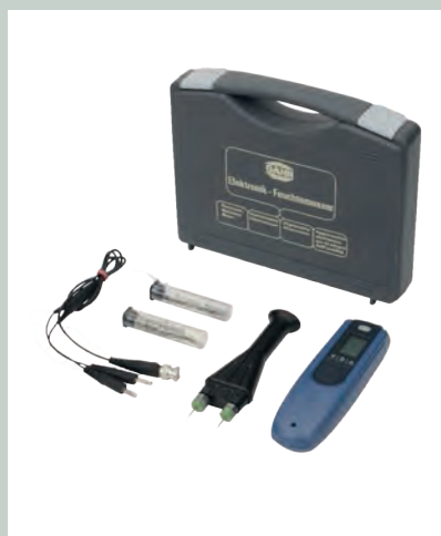
SET 1 contains the M 20 drive-in electrode
